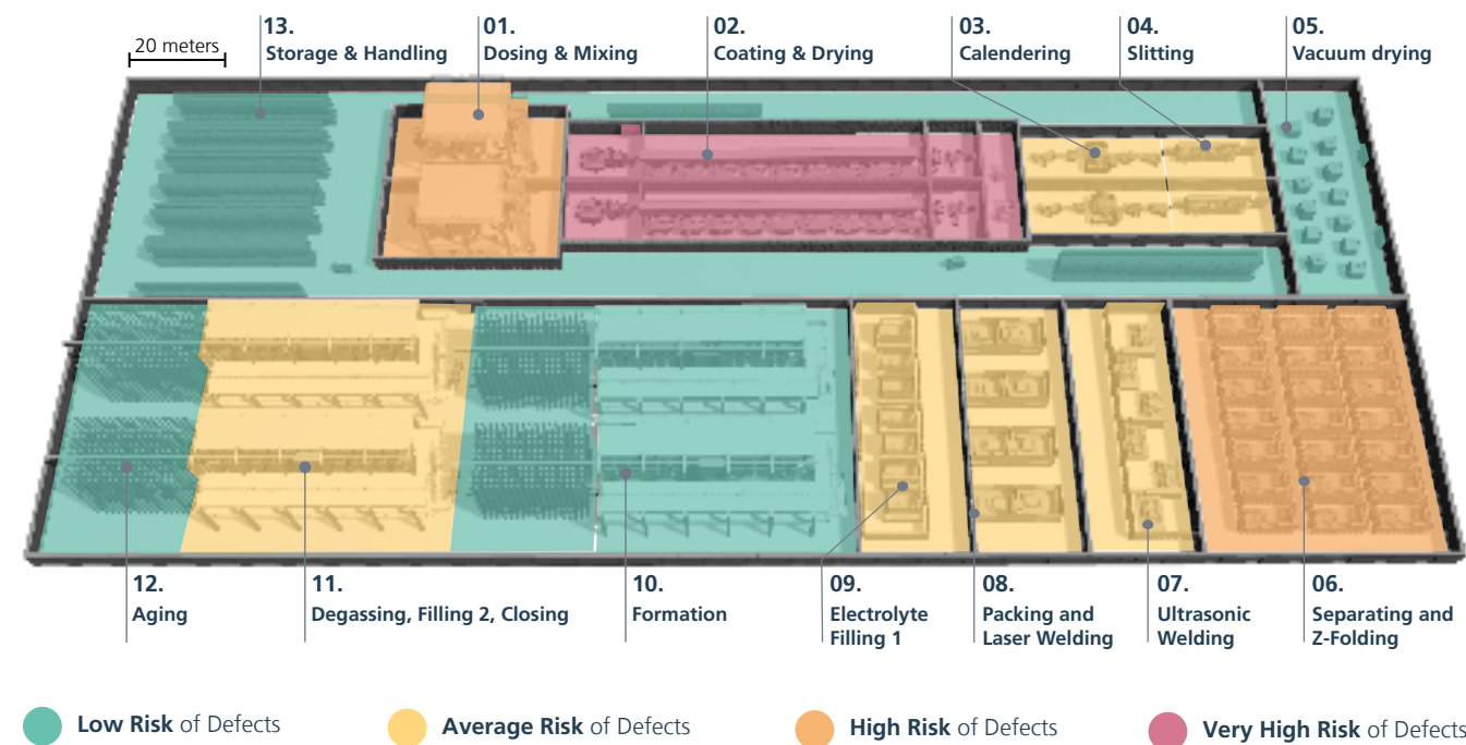
Figure 6 Layout of a typical, modular battery cell production line (7-10 GWh/a) and their risk level for defects. A battery cell factory has multiple of such modules/lines.
